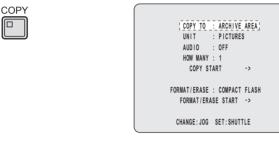
**3** Turn the jog dial to select "FORMAT/ ERASE", and then turn the shuttle dial clockwise.
